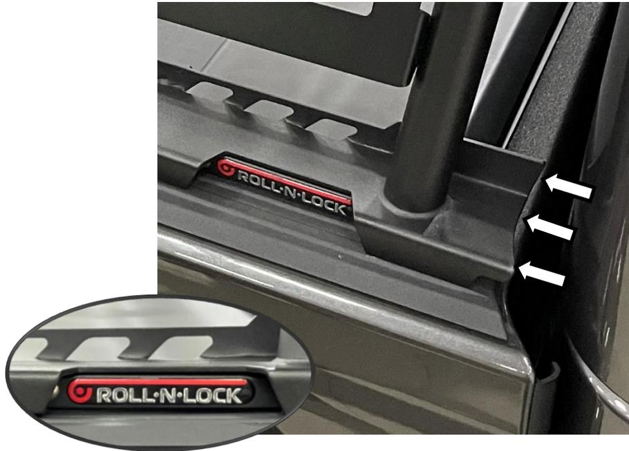
**Step 3:** Slide (x6) threaded channel nuts through rear opening of the T-slotted bed rail and align with the mounting holes in the Sport Bar.
